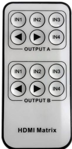
**OUTPUT A:** Press IN1\IN2\IN3\IN4 button will fast switch to select input source to HDMI OUTPUT A, and the LED will indicate the corresponding input source. Press ◀ ▶ button OUTPUT A will cycle from input IN1\IN2\IN3\IN4.
